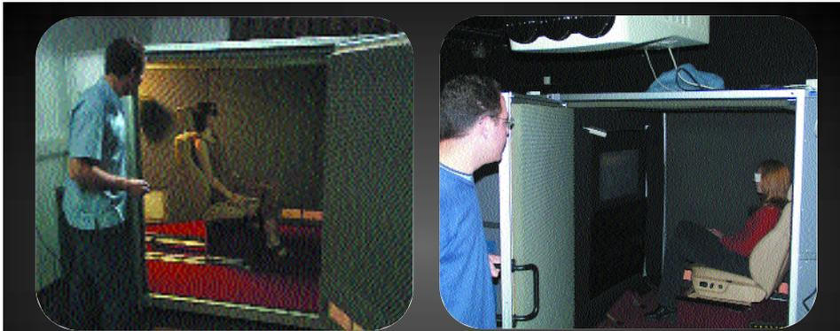
The ITC's Platform for Immersive Television (PiT) *in situ* at the Immersive Television Laboratory at Goldsmiths College. The PiT is a controlled test environment, but replete with a widescreen, 3-D display, adjustable seat and surround sound, it can already give viewers an immersive TV experience. Its prime function, however, is as a test bed for experiments designed to identify which display parameters optimise immersive television
